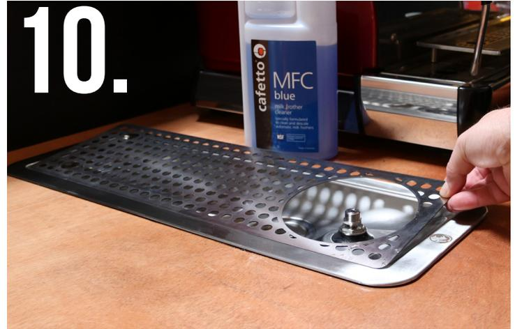
Reassemble the Drain Tray,
