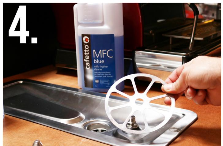
4. Remove the Actuator Plate.
