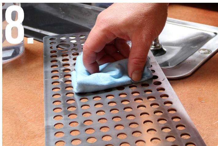
8. Built-up solids may need mechanical/hand agitation to remove.
