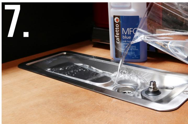
7. Pour the remaining diluted solution into the rinser slowly and allow the solution to drain. This will clean the drain piece and drain hose.
