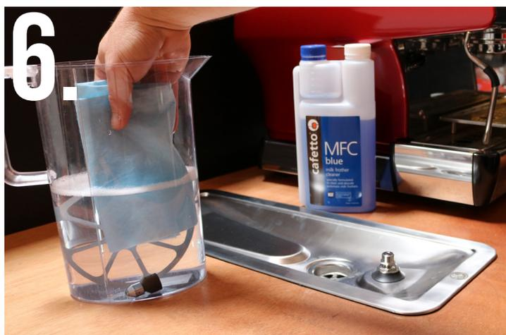
6. Dip a soft cloth into the diluted cleaning solution and use to wipe down the surfaces of the rinser. Remove soaking parts from cleaning solution and rinse.
