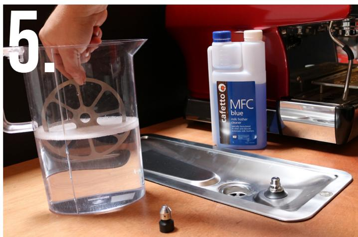
5. Add the removed parts to the Daily Milk Frother Cleaner solution. Allow the parts to soak while cleaning the remainder of the rinser.
