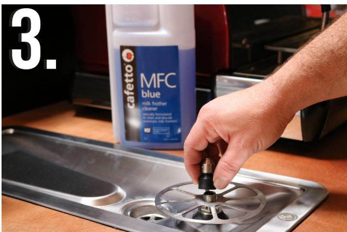
3. Unscrew the spray valve from the rinsler body.
